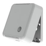
4. Attach the sensor part to the back panel.
