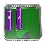
2. **Install the batteries.** The ERS requires one or two AA batteries. The battery type is **3.6V** Lithium Battery *110529-batt*. Use battery slot A if only one battery is used. The number of batteries, 1 or 2, depends on the model.
